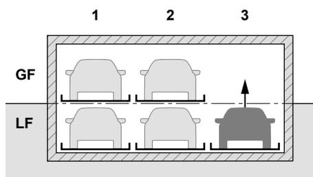
The empty space is now located above the vehicle being removed. The parking space in **grid 3/LF** is raised.
