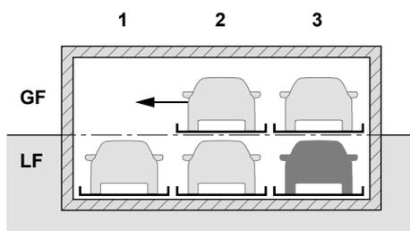
To remove the vehicle from the space in **grid 3/LF**, the GF platforms are moved to the left.
